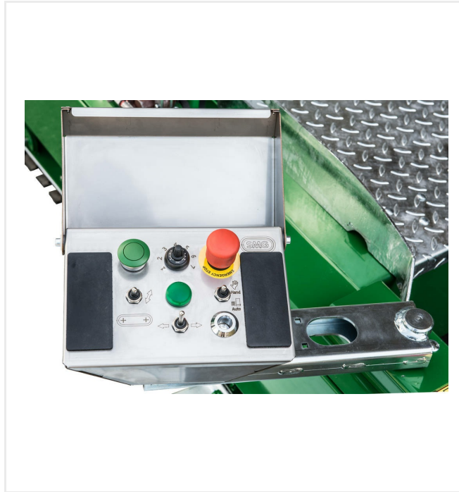
Detachable control panel for left and right
