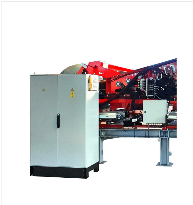
Switch box with controls
