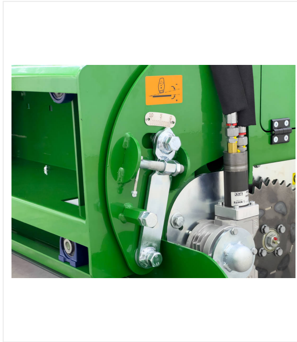
Adjustment of compaction
