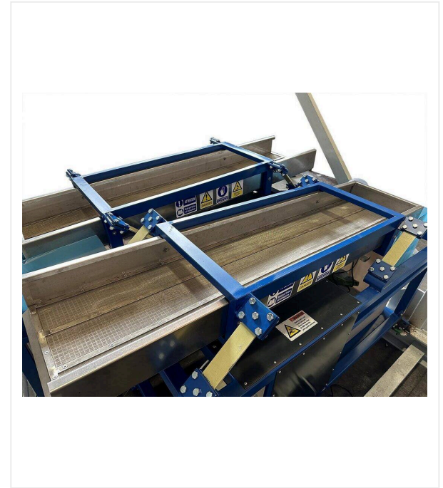
Vibration dewatering system
