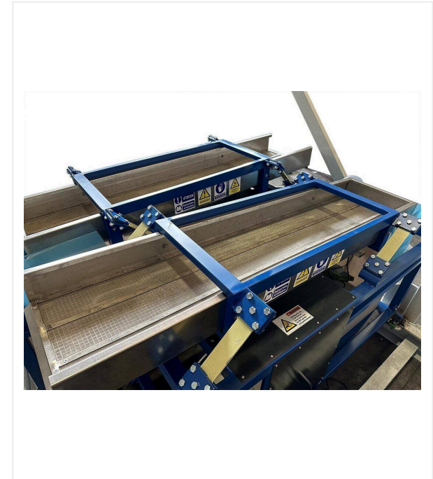
Vibration dewatering system
