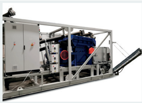
Control and operating unit Central unit (left) and control unit for fiber and filament separators (right)
