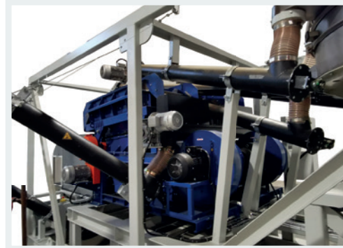
Separation units Precision aggregates for the separation of sand and rubber granulate according to grain size and density
