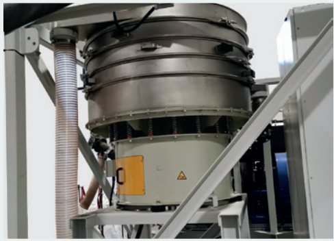
Tumbler screening plant Mechanical pre-separation by tumbler screen – ensures process stability and reliably removes coarse contaminants
