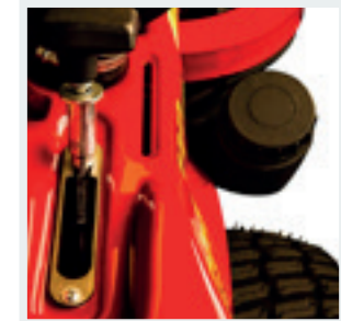
REFUELING Fuel tank neck outside for 16 liter fuel tank.
