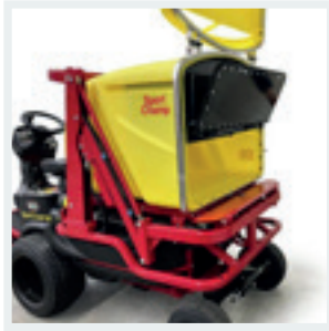
NEW EQUIPMENT Filter box with larger capacity, automatically cleaning filter and self closing tailgate.
