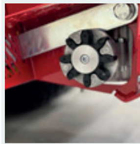
COUPLING PTO to power the attachments.
