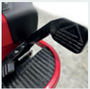
PEDAL Infinitely variable hydrostatic drive.
