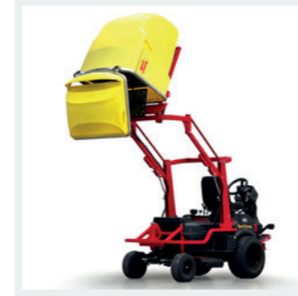
HYDRAULIC LIFTING OF CONTAINER Allows comfortable emptying in containers.
