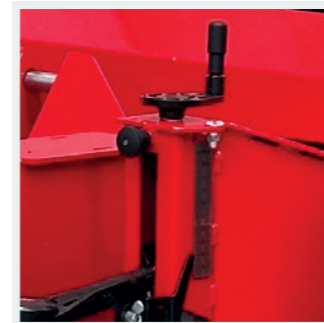
FUNCTIONAL Working depth adjustment, adjustment spindle, height indicator, spirit levels.
