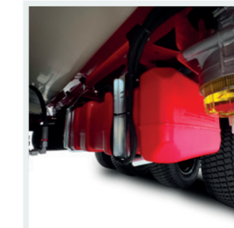
FUEL TANK 53 liter fuel tank for maximum range.
