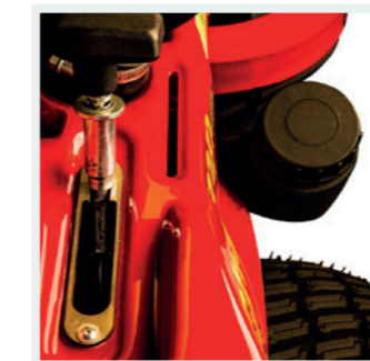
REFUELING Fuel tank neck outside for 16 liter fuel tank.
