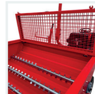
EFFECTIVE Four hydraulically driven paddle shafts within the container keep the infill material loose and ensure a consistent distribution.
