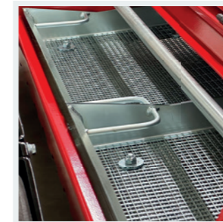
VARIABLE Continuously adjustable vibrating screen (now without drive shaft).
