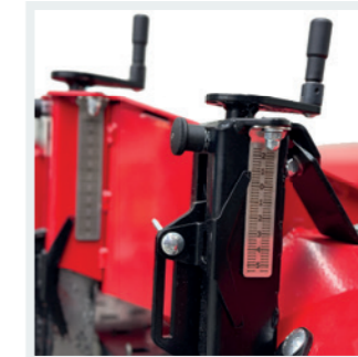
EFFECTIVE Spring tines with adjustable working depth for loosening the bedding material.
