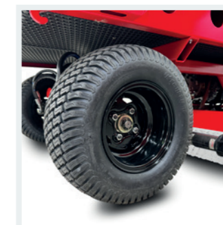
LIGHT-FOOTED Four large-volume turf tires for minimal surface pressure.
