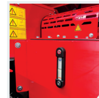
REFUELLING Diesel tank with fuel gauge.
