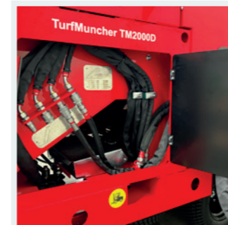
HYDRAULICS QUICK COUPLINGS for the drive of conveyor belt.
