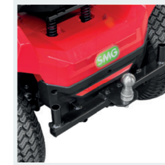
HITCH For drag mats, triangle brushes and magnet bars.
