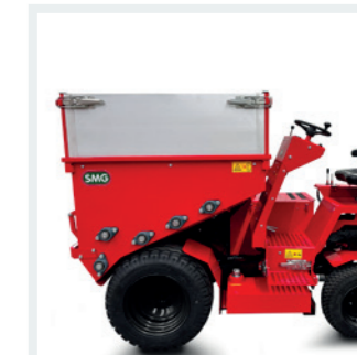
SINGLE SIDE WALL Material container that has a capacity of 800 liters, which can be expanded up to 3000 liters by attaching aluminum extension frames.
