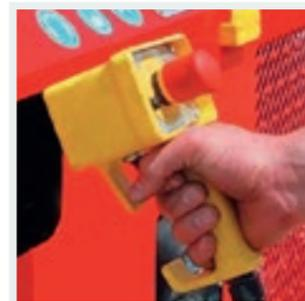
**B1505 ECO:** Cabel handsteering for controlling the infilling process and driving direction. Range up to 5 m (B1505 ECO).
