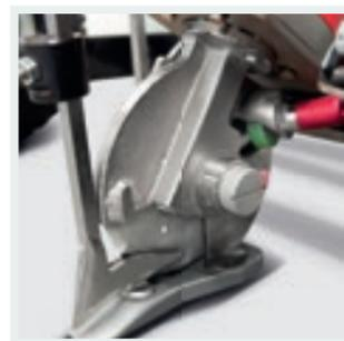
**CUTTING:** Sharpening system for cutting blades.
