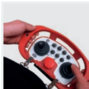
**COMFORTABLE:** Radio frequency (RF) remote control for handling all functions, with a range of 100 m (B1505RC).
