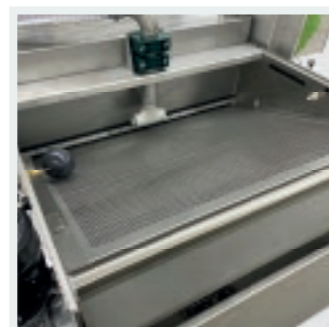
Belt filter with tear-resistant filter fleece (120 µm) including collecting container with float switch
