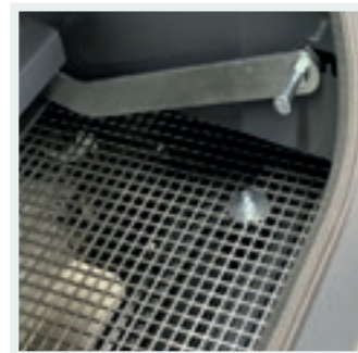
VERSATILE: Material flap to adjust the flow of debris and infill.
