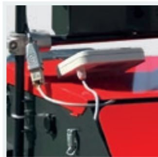
EASY HANDLING: Operation via hand- or radio remote control.
