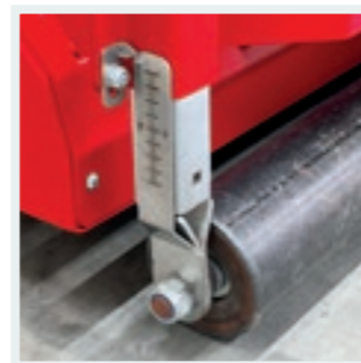
CONTROL: Scale to control working depth and level.
