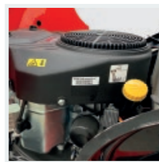
Petrol engine 12.2 kW (16.6 HP)
