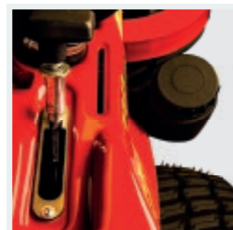
REFUELLING: Filler neck outside for 30 liter fuel tank.
