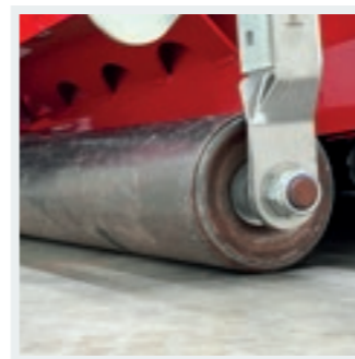
GENTLE: Roller for minimum ground pressure.
