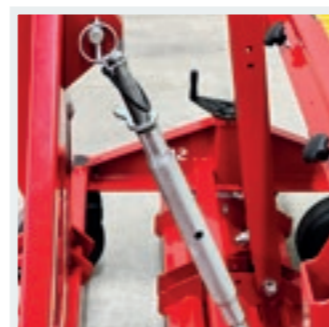
STRONG: Linkage for the use with three point hitch.
