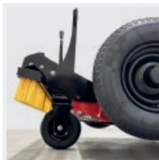
ONE OF A KIND: Fold-out transport rollers for transverse drive through doors and thigh gates.
