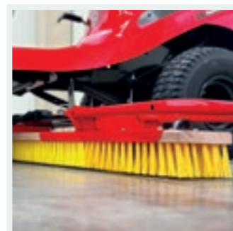
COMBINATION: Tines and drag brushes adjustable.
